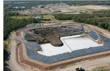
Aerial view of the cell – 12/4/23. Note that fluffy layer material has been pushed over the bund from the NE to NW quadrants.
