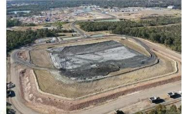
Aerial view of the cell – 11/8/23. Waste is now 4m below design height or 17m thick in total (9m below the batter and 8m above the batter).
