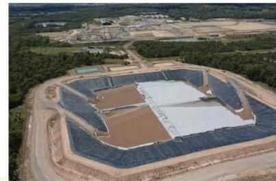
Aerial view of the cell – 6/2/22. Cell complete and ready to receive waste. This has now started in the SE quadrant as @ 13/2/23.
