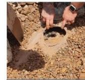
Figure 17. 100mm Puncture in NE Cell Floor (S2, A2)
