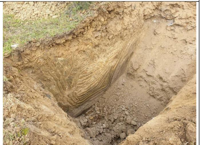
**Photograph 58:** AEC 33 Area East of the Clay Borrow Pit AECBP\_TP14. Foreign material observed.
