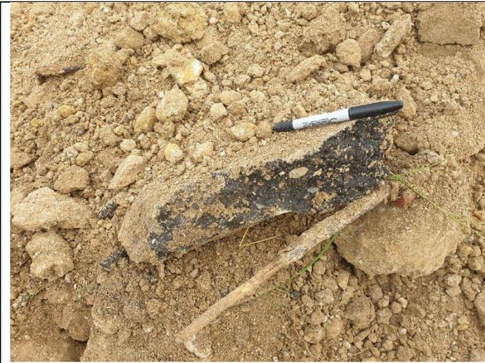
**Photograph 61:** Asphalt in test pit spoil AECBP\_TP14.
