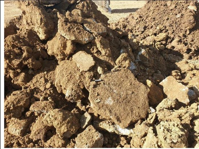
**Photograph 37:** Large concrete boulders in test pit spoil AECBP\_TP3.
