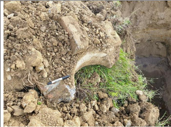
**Photograph 49:** Large boulders and brick in test pit spoil AECBP\_TP10.
