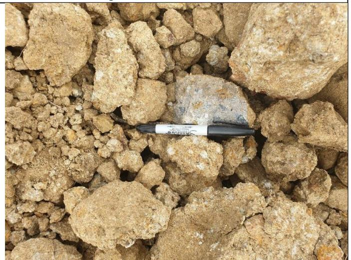
**Photograph 60:** Concrete boulders in test pit spoil AECBP\_TP14.
