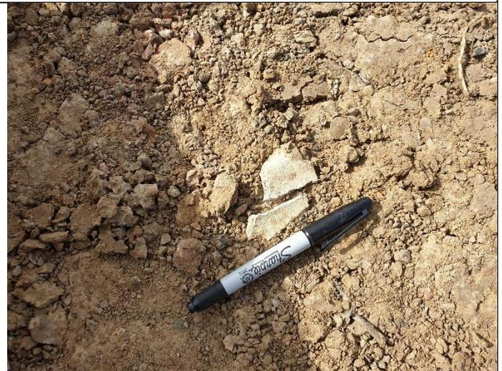
**TP66:** AEC 33 Area East of Clay Borrow Pit ACM fragment identified at surface of undisturbed soil.
