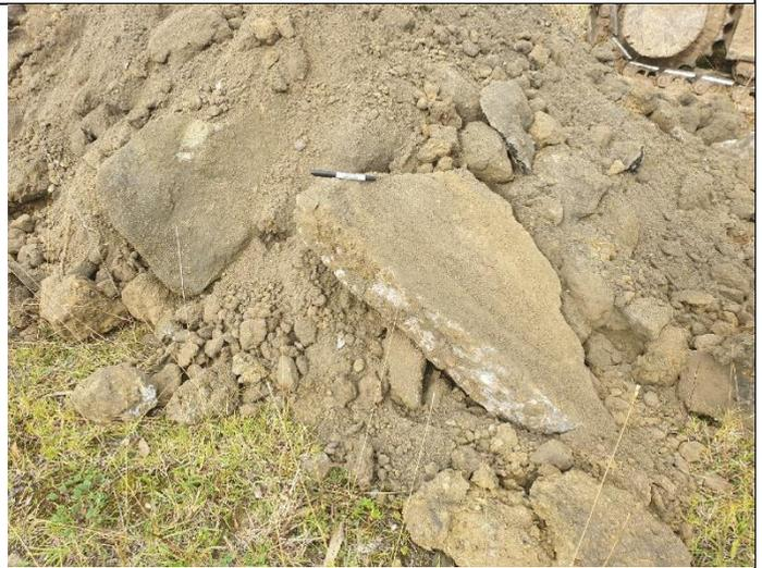
**Photograph 54:** Large Boulders in test pit spoil AECBP\_TP13.
