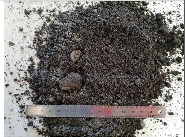
**Photograph 30:** AEC 18 Pot Rebuild Area 77A-Pit 3 slurry from concrete core cutter.
