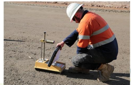
PRC • ECC Works – Compaction testing of perimeter road select fill layer by HILF density measurement (6/7/21)
