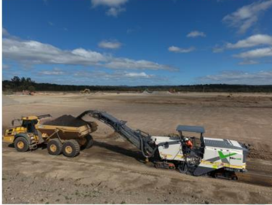
Asphalt milling machine removing asphalt road surfaces
