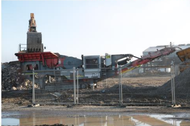
CRUSHING PROSPEROUS FUTURES Jaw crusher in Carbon Plant Area. Approximately 202,000 tonnes of concrete has now been crushed for recycling back on site.
