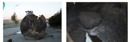
UST for petrol turned out to be previously decommissioned and filled with sand. Letter from Ramboll on UST decommissioning received. Certificate of destruction received from scrap metal recycler (4/8/20)
