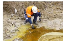
Sampling by Ramboll to determine nature of hydrocarbon contaminants (29/11/19)
