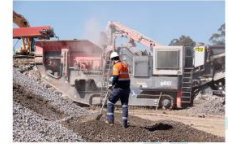
CREATING PROSPEROUS FUTURES Ramboll continuing to sample concrete stockpiles for % foreign material content (5/9/19)
