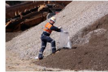
CREATING PROSPEROUS FUTURES Ramboll continuing to sample concrete stockpiles for % foreign material content (5/9/19)
