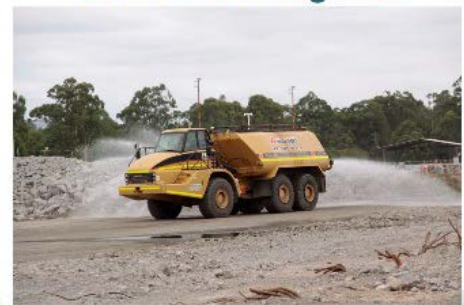
Moxy watercart now on site for additional dust suppression (14/2/2019)
