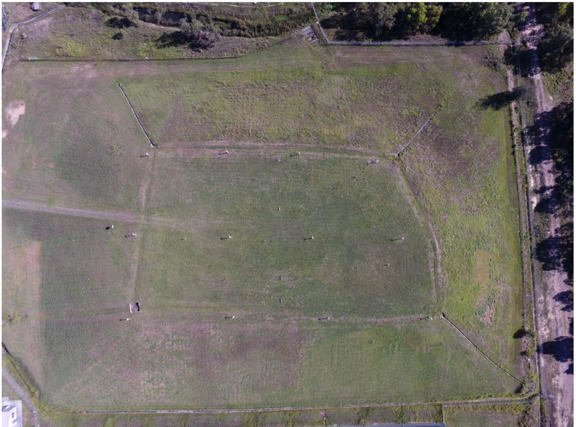
Figure 2 Birdseye view of capped waste stockpile
