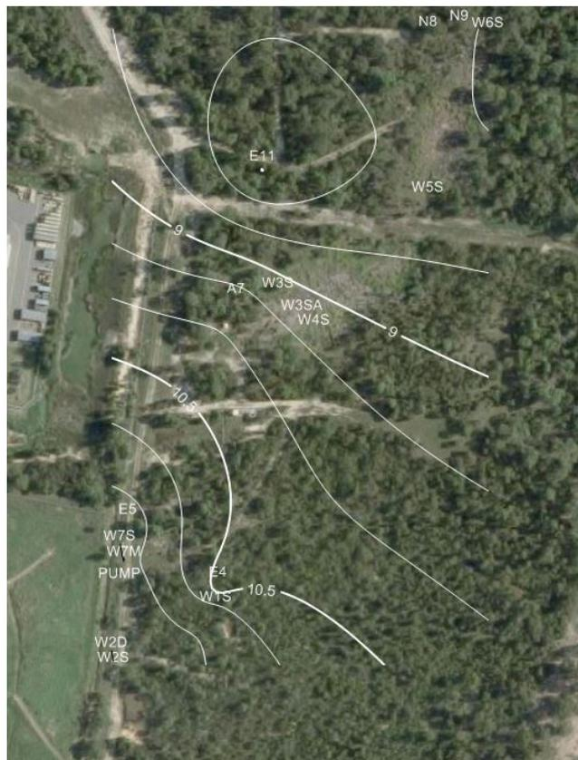
Figure 10: February 2014 Shallow Groundwater Flow Direction
