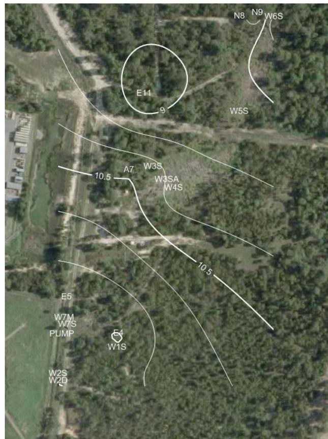
Figure 14: June 2015 Shallow Groundwater Flow Direction
