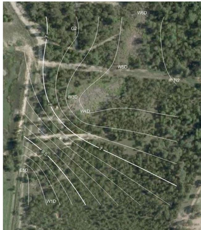
**Figure 21: July 2013 Deep Groundwater Flow Direction**
