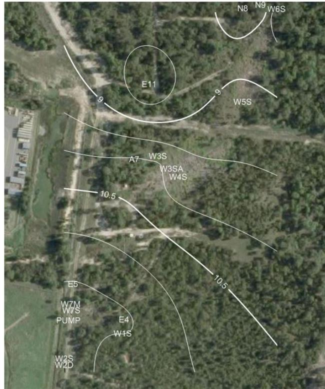
Figure 15: September 2015 Shallow Groundwater Flow Direction
