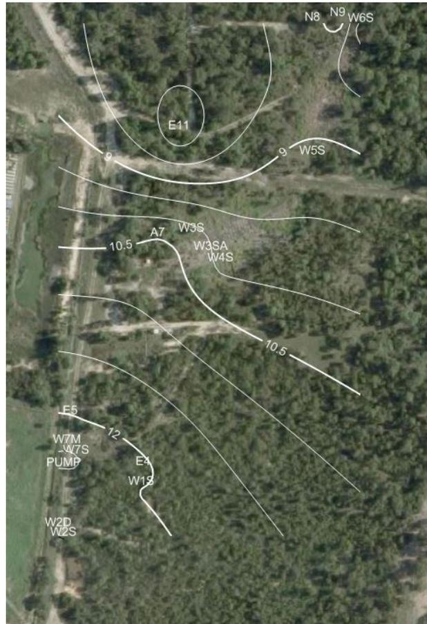
Figure 9: November 2013 Shallow Groundwater Flow Direction
