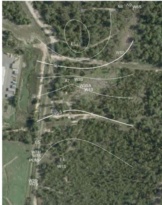
**Figure 11: June 2014 Shallow Groundwater Flow Direction**
