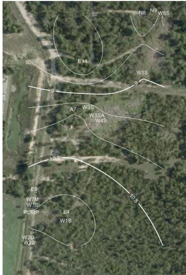
Figure 13: February 2015 Shallow Groundwater Flow Direction
