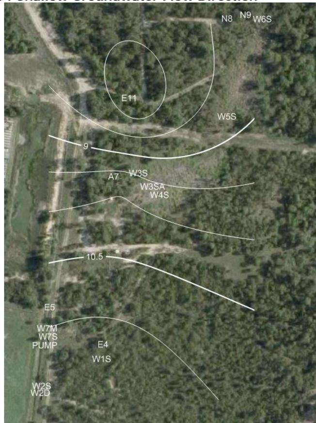
**Figure 12: November 2014 Shallow Groundwater Flow Direction**
