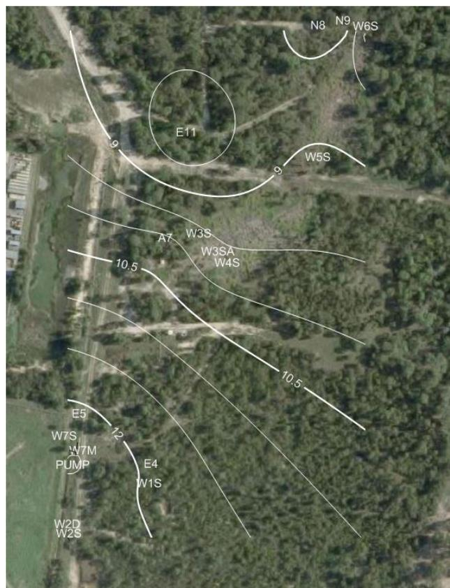
**Figure 8: July 2013 Shallow Groundwater Flow Direction**
