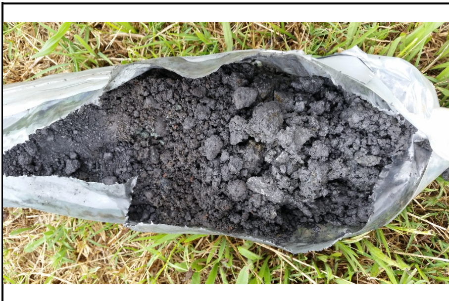
Photo 6: Waste material encountered from approximately 11.5 to 12.0 mbgs. Waste at approximately 11.8 mbgs was noted to be wet.
