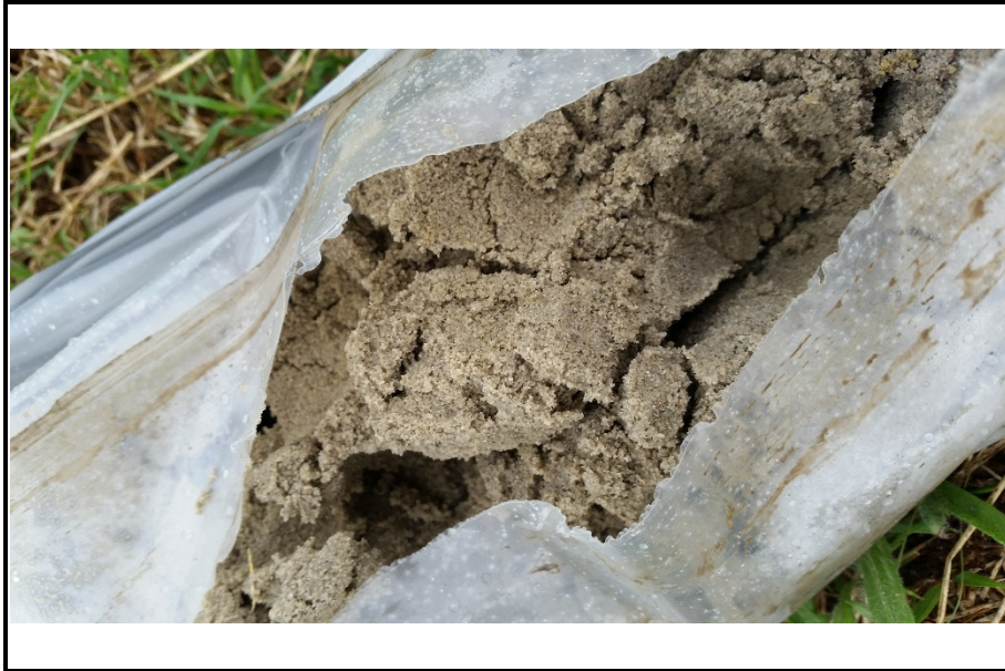
Photo 7: SAND encountered beneath capped waste at borehole location MW206
