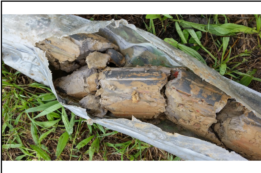
Photo 2: CLAY encountered beneath capped waste at borehole location MW202
