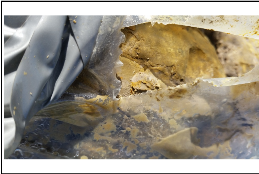
Photo 5: Sandy CLAY encountered beneath capped waste at borehole location MW203
