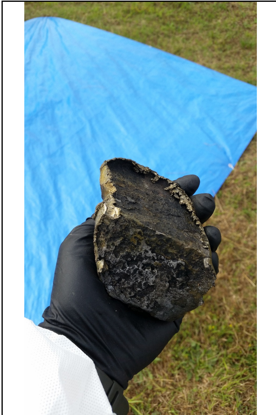
Photo 3: Steel encountered at borehole location MW202.
