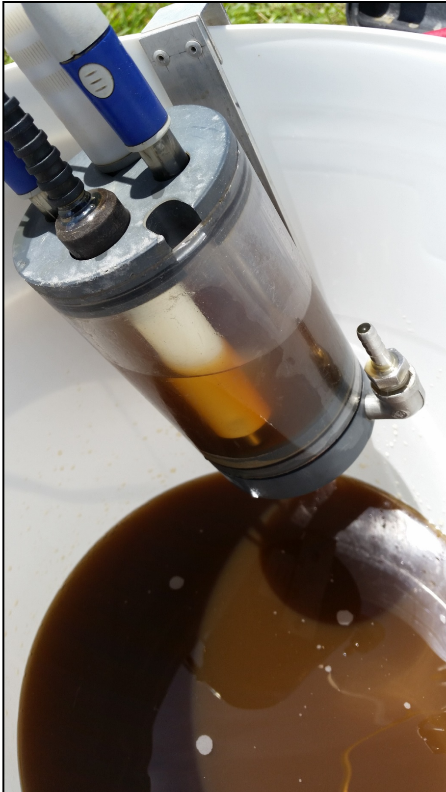
Photo 9: Leachate encountered at location MW203
