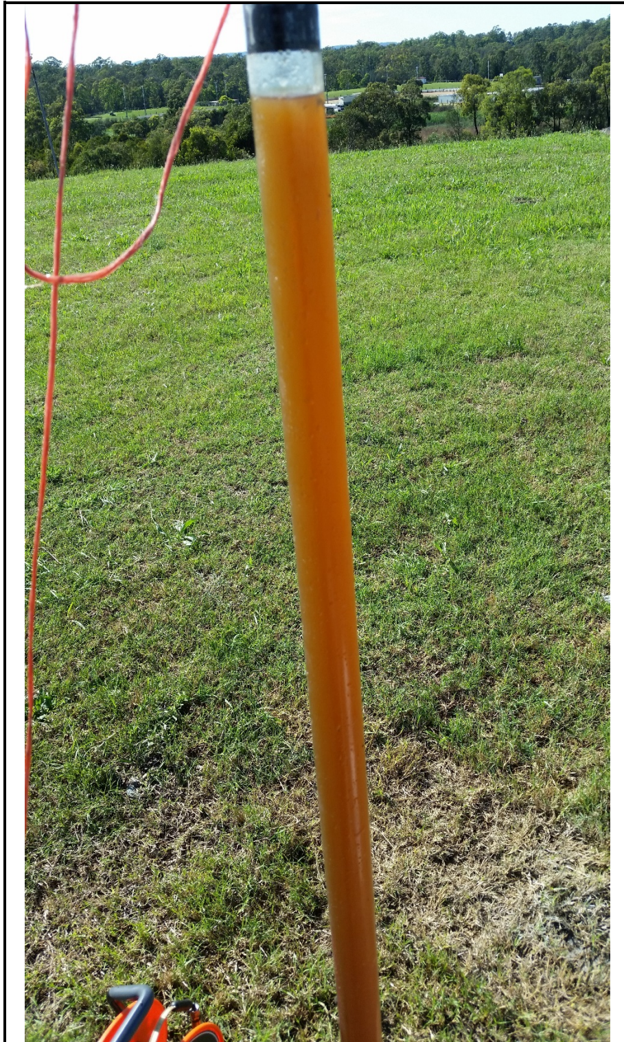
Photo 8: Leachate encountered at location MW206
