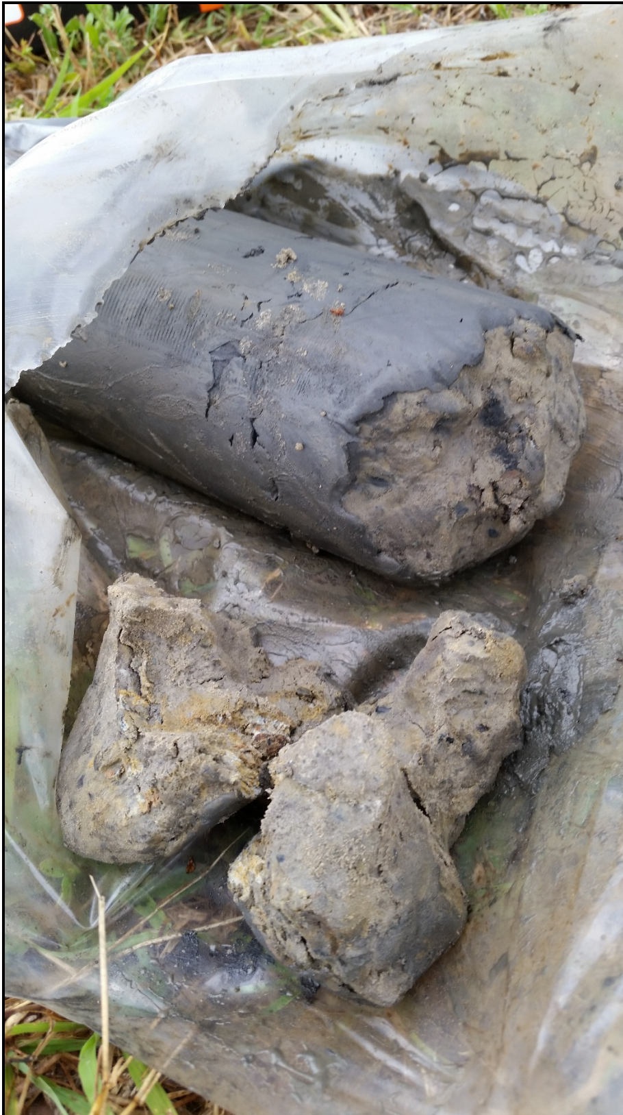
Photo 1: Sandy CLAY encountered beneath capped waste at borehole location MW201
