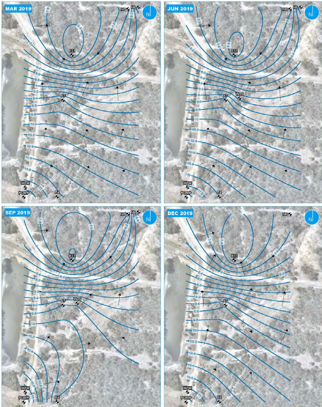
Aerial photography by Heamap, flown 20.12.2019 Legend ↕ Monitoring location → Flow direction — 0.2 m water level contour
