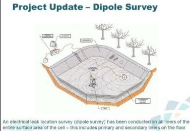
An electrical leak location survey (dipole survey) has been conducted on all liners of the entire surface area of the cell – this includes primary and secondary liners on the floor and the primary liner on the sidewalls of the cell. It's purpose is to pick up handling damage caused by deployment of sand, drainage aggregate and the soil confining layer.
