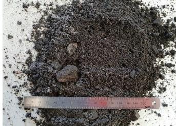
**Photograph 30:** AEC 18 Pot Rebuild Area 77A-Pit 3 slurry from concrete core cutter.
