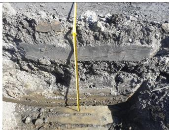
**Photograph 8:** AEC 2 Anode Waste Pile TP206. Water at base of excavation.
