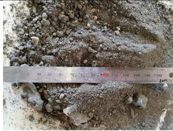
**Photograph 28:** AEC 18 Pot Rebuild Area 77A-Pit 2 slurry from concrete core cutter.
