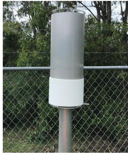
Photo 41 – Dust Gauge located near Speedway (DDG1) – fenced and with hard case to protect from vandalism.
