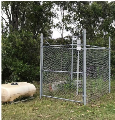
Photo 41 – Dust Gauge located near Speedway (DDG1) – fenced and with hard case to protect from vandalism.
