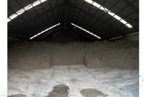
West Surge Pond sediment with 4% cement (1/10/21)
