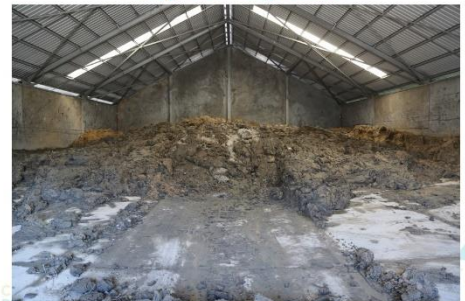
West Surge Pond sediment – 2% cement trial (23/9/21)
