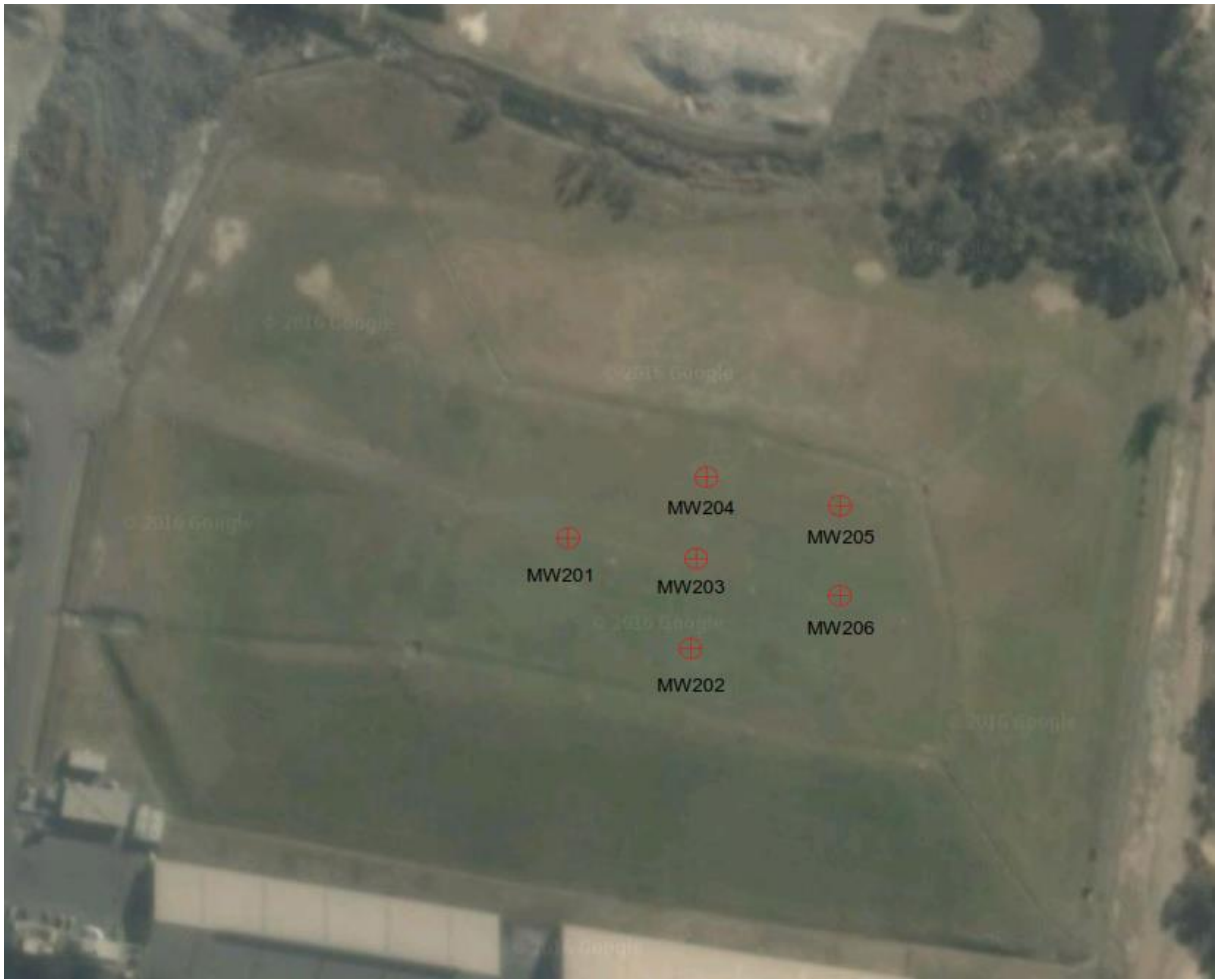
Figure 2 Capped waste stockpile sampling wells (per Ramboll Environ)
